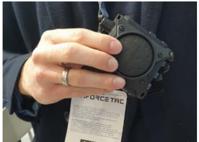
The CT-MultiPTT 3C is a central operation and control unit that can simultaneously coordinate three independent communications circuits. (Photo: Mönch Publishing/Stefan Nitschke)
