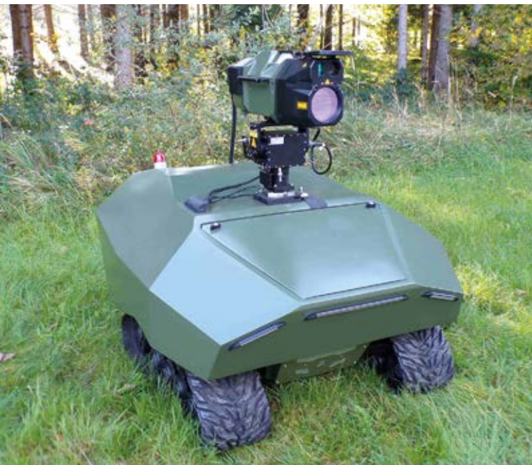
With MILOS-D, the MBDA engineers developed a laboratory prototype of a small portable laser especially for the army and police. Photo: MBDA Deutschland
