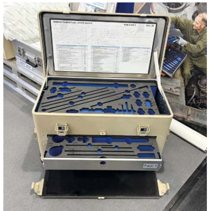
A collaboration with the German Armed Forces. A Base for the armorer's toolbox: special tools can be individually configured and organized, for example, by weapon group.
